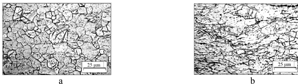
Fig. 3. Microstructure of MgCa0.8 for temperature 200 °C and tool velocity 60 mm/min correspond to fig. 3, b:
